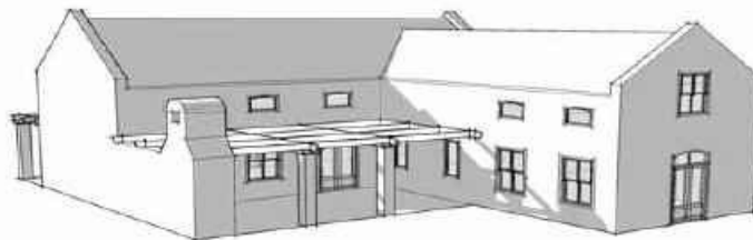
Figure 6: Core building with double pitched roof and gable end walls
